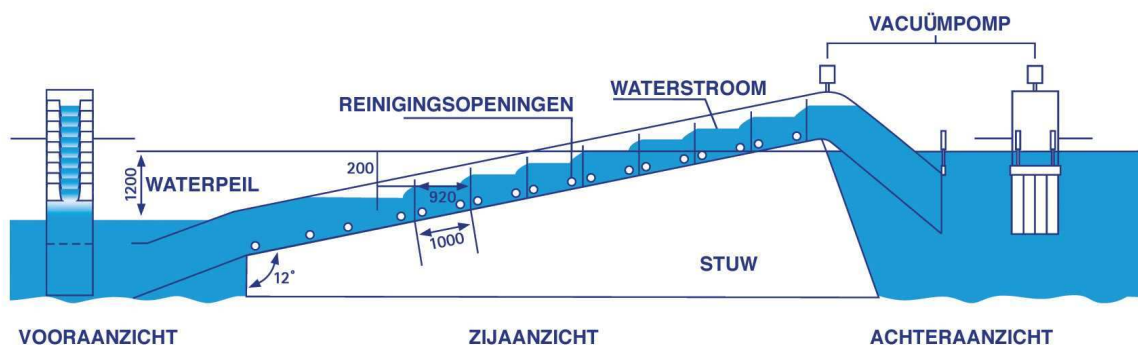
Figuur 5.12 De FishFlow hevelvistrap (bron: www.fishflowinnovations.nl ).
